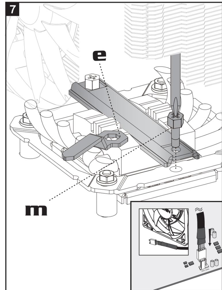
⊕ Screwdriver with length longer than 160mm
